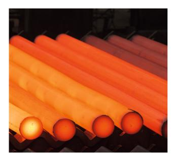
Our rolled products are divided into two categories according to the mill in use. The medium section mill provides the round, square bars up to 75 mm and the flat and hexagonal bars up to 71 mm. The large section mill provides the square, round bars above 75mm and large flat bars.
